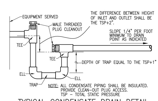
TYPICAL CONDENSATE DRAIN DETAIL DRAW THROUGH UNIT NOT TO SCALE
