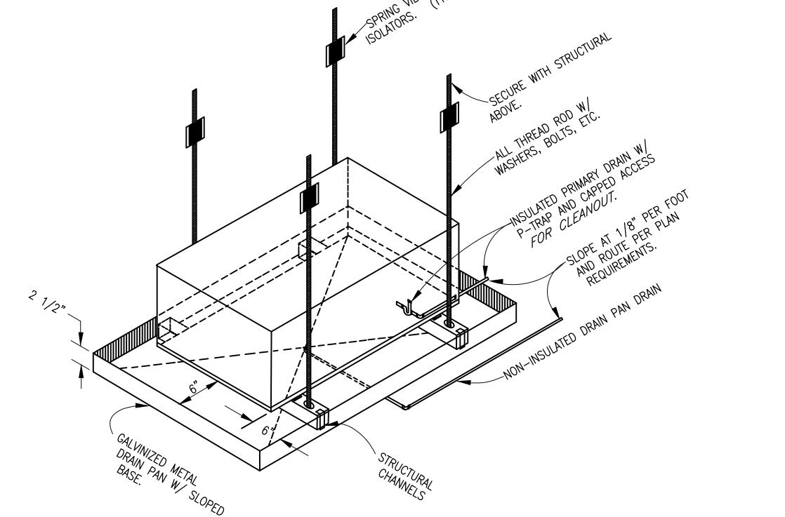
TYPICAL HORIZONTAL ERV DETAIL NOT TO SCALE
