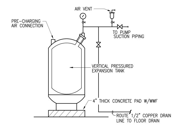
EXPANSION TANK DETAIL NOT TO SCALE
